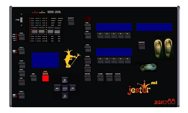
The JesterML lighting desks are compact user-friendly memory desks which record channel levels and fixture information, and provide both theatre style sequential memory access and sub-master style access, as well as colour, beamshape and position palettes.
